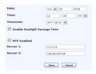
The time/date on the Dualcom S can either be set manually or automatically using NTP.
